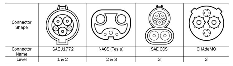
Nearly all EVs in North America use either the SAE CCS or NACS (Tesla) connector types for level 3 charging. Throughout 2024 the NACS connector became the dominant connector type amongst EVs as most major vehicle manufacturers adopted the NACS connector. Adapters allow many vehicles to utilize both the SAE CCS and NACS connector types. The CHADeMO connector is uncommon in 2025.
